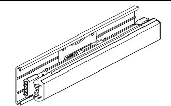
4. The fixture can be rotated to achieve the desired angle. Grab the fixture, and carefully push down to disengage the teeth. Then, rotate the fixture in desired angle and position. For the 48 in. model, match the angle of rotation for both mounting brackets.
